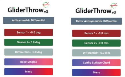
When you are trimming or calibrating a Symmetric Flight Control, like the flaps you want both sides control surfaces deflect the same: Symmetry in an airplane is critical for stable flights... Then the standard page is ideal it will show the difference in reading of the two sensor: Remember sensor 2 minus sensor 1.
