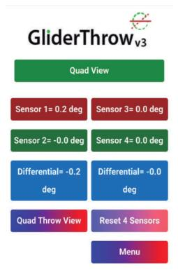
In this Screen you can check the reading of four sensors and perform any adjustment in your plane for instance if your reference information is in degrees or if you want to do so.
