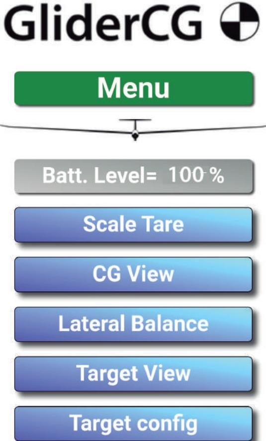
The first menu option "**Scale Tare**" allows you to zero the weight measurement or tare the scale.
