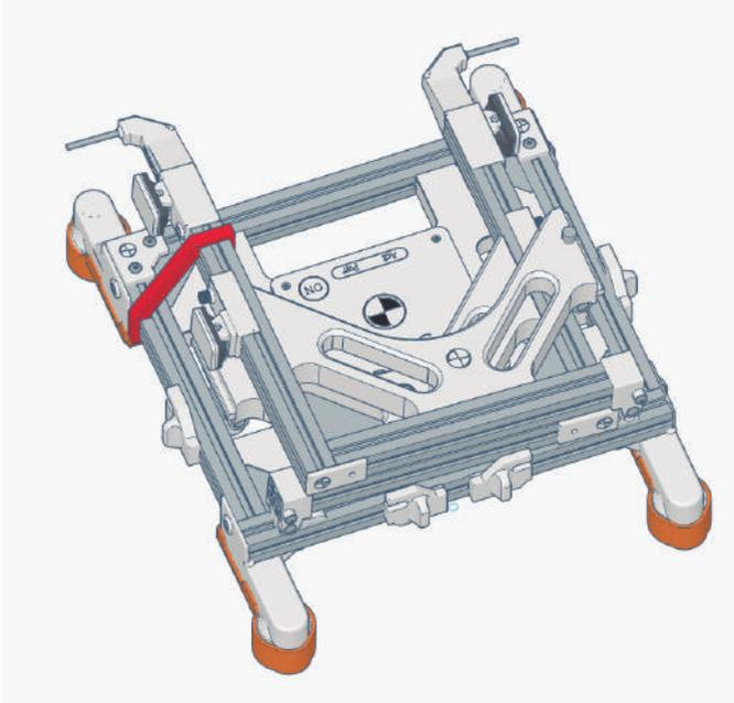
Before starting remove the protectors that cover the legs of the device and protect the sensors from impacts.
