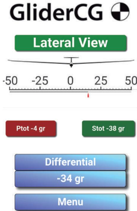
The numbered rule in the upper part will help us to identify in a simple way the weight deviation between both sides
